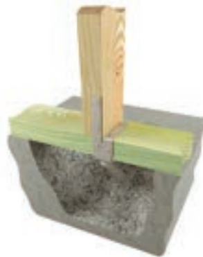
Typical FA3 one-tab-up installation
