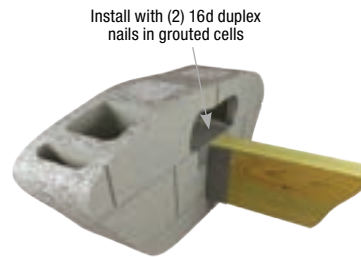
Typical MPH double-ply installation
