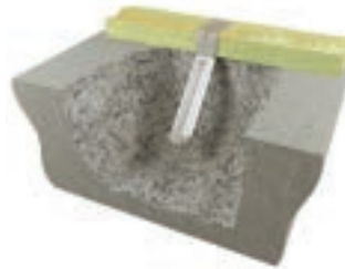
Alternate FA3 installation (concrete slab only)
