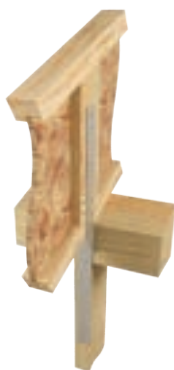
Typical MTW20 I-joist rafter installation
