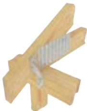
Typical RT7A truss/rafter to double plate installation
