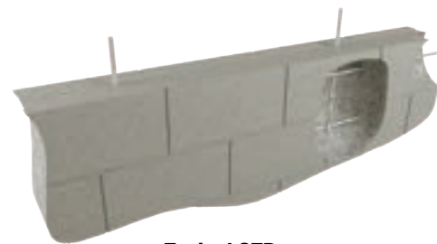
Typical STB concrete block installation
