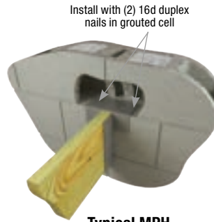
Typical MPH single-ply installation
